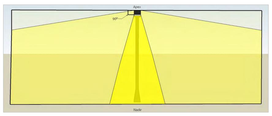
Figure 3: Full Cut-off Fixture
