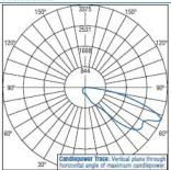
Independent Testing Laboratories certified test, Report No ITL68359, Candlepower trace of 6000K, 40 LED LEDway Streetlight luminaire with IESNA Type III Medium distribution w/ backlight control. Luminaire with 5,084 initial delivered lumens operating at 700mA. All published luminaire photometric testing per med to IESNA LM-79-08 standards.
