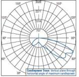
Independent Testing Laboratories certified test. Report No. ITL68859. Candlepower trace of 4300K, 40 LED LEDway Streetlight luminaire with IESNA Type III Medium distribution w/ partial backlight control. Luminaire with 5,440 initial delivered lumens operating at 700mA. All published luminaire photometric testing performed to IESNA LM-79-08 standards.
